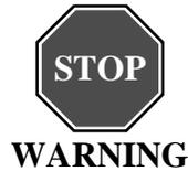
**When wearing a Conductive Wrist Strap, be careful near sources of high voltage. The low impedance provided by the wrist strap also increases the danger of lethal shock from accidentally touching high voltage sources.**
