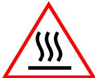
This graphic symbol appears in this manual and on the station front panel (and other station surfaces) as a reminder that the station can become extremely hot during normal station operation. Turn off all power to the station, and wait until sufficiently cool before touching the station.
